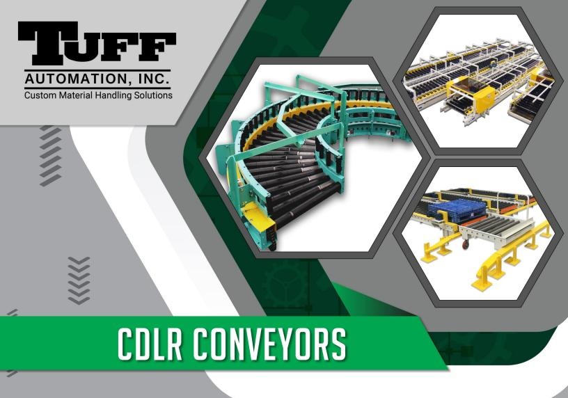
The robust design of our chain driven live roller (CDLR) conveyors makes them perfect for transporting heavy items such as loaded pallets, tires, and barrels. In our CDLR conveyor, each steel roller is driven by chains running from roller to roller over sprockets. Rollers are held in place between two steel frames by either internal springs or retaining pins.
